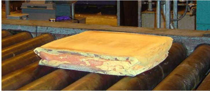
Figure 3.7: Ti64+1B billet after first round of 8 rolling passes. Ref: Tamirisakandala.
