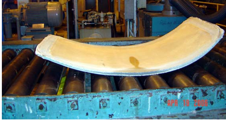
Figure 3.9: Ti64+1B plate after third round of 8 rolling passes. Ref: Tamirisakandala.
