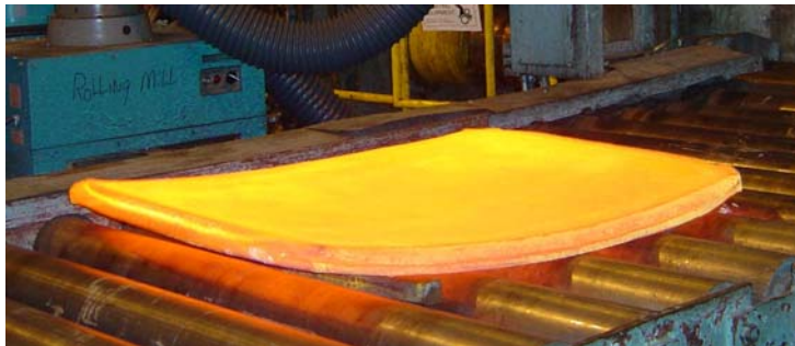
Figure 3.8: Ti64+1B, now a plate after second round of 8 rolling passes. Ref: Tamirisakandala.
