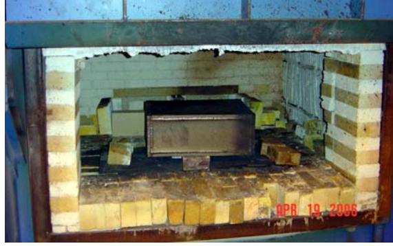
Figure 3.5: Ti64+1B billet being loaded into furnace. Ref: Tamirisakandala.
