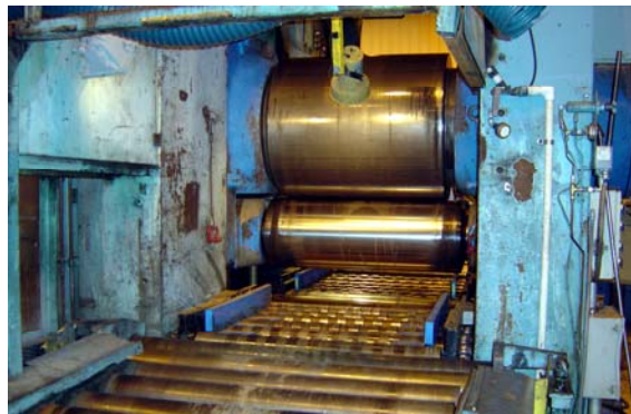
Figure 3.4: Rolling mill at Oakridge, TN facility. Ref: Tamirisakandala.
